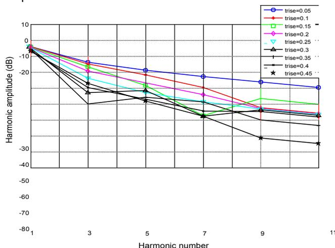
Figure 16. Harmonic EMI reduction as a Function of Slower Rise/Fall Time
