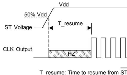
Figure 5. Standby Resume Timing ( ST Mode Only)
