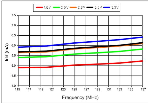
Figure 8. I<sub>dd</sub> vs Frequency
