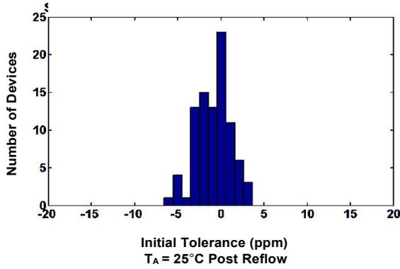
Figure 5. Initial Tolerance Histogram
