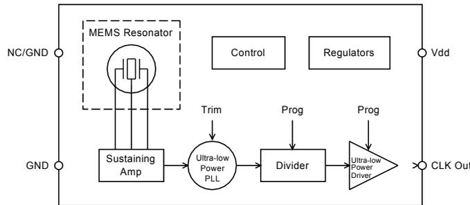
**Figure 3. JYJE1630 Block Diagram**
