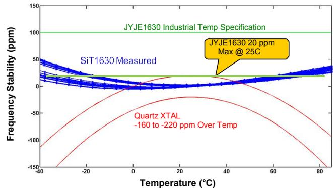
Figure 4. JYJE vs. Quartz
