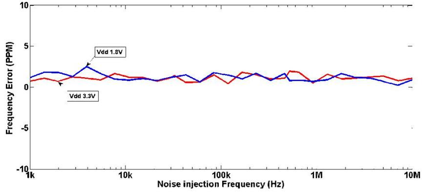
Figure 9. Power Supply Noise Rejection ( $\pm 150\text{mV}$  Noise)
