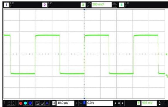
Figure 10. LVC MOS Output Waveform
