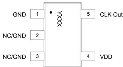
**Figure 1. Pin Assignments**
