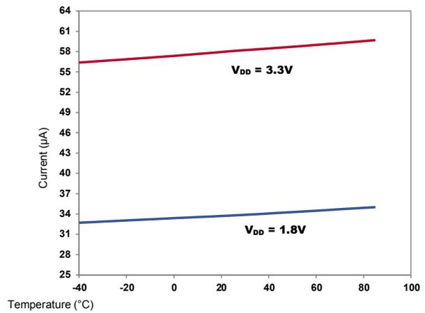
Figure 12. Supply Current vs Temperature (F<sub>OUT</sub> = 2 MHz)
