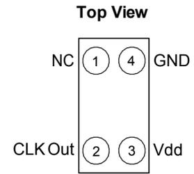
**Figure 1. Pin Assignment**
