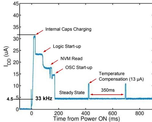
Figure 4. Start-up and Steady-State Current Profile
