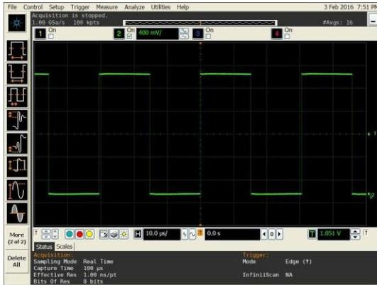
Figure 3. LVC MOS Output Swing ( $V_{DD} = 1.8\text{V}$ )
