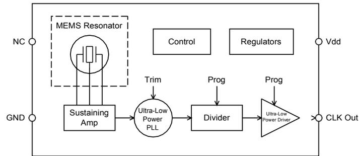
Figure 2. JYJE1533 Block Diagram
