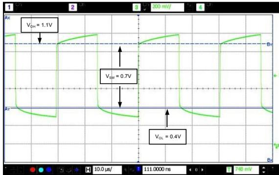
Figure 13. NanoDrive™ Output Waveform ( $V_{OH} = 1.1\text{V}$ ,  $V_{OL} = 0.4\text{V}$ ; JYJE1533AI-H4-D14-32.768)
