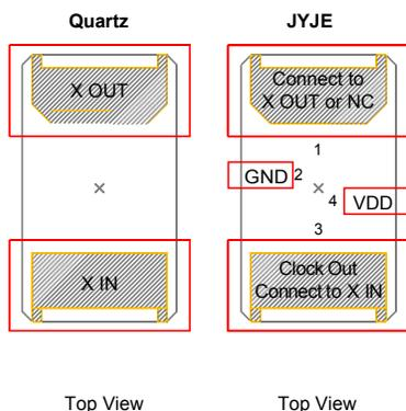
Figure 3. JYJE1533 Footprint Compatibility with Quartz XTAL Footprint<sup>[6]</sup>
