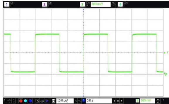
Figure 14. LVC MOS Output Waveform ( $V_{swing} = 1.8\text{V}$ , JYJE1533AI-H4-DCC-32.768)
