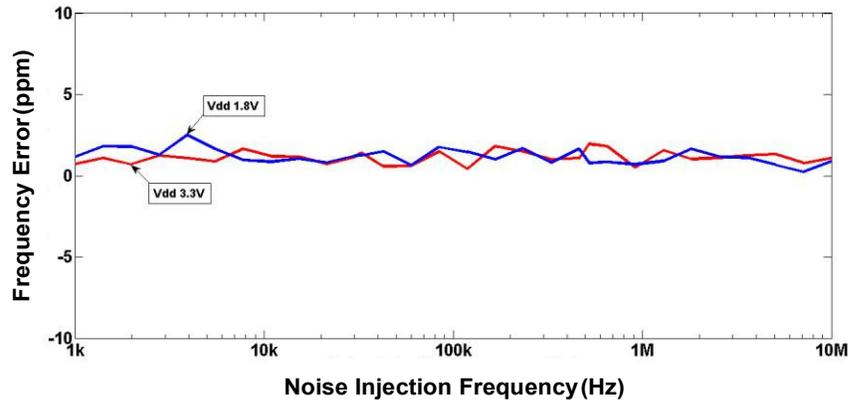
Figure 12. Power Supply Noise Rejection ( $\pm 150\text{mV}$  Noise)
