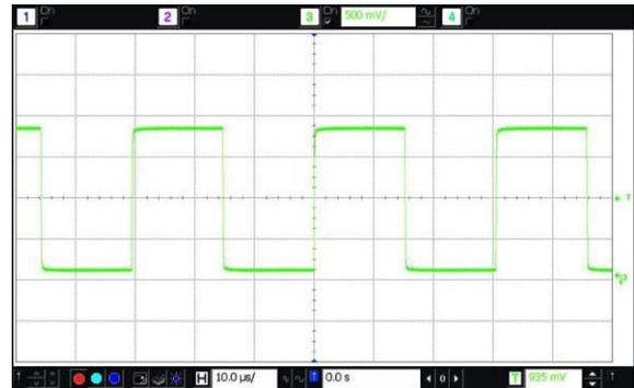
Figure 6. LVC MOS Waveform (Vdd = 1.8V) into 15 pF Load
